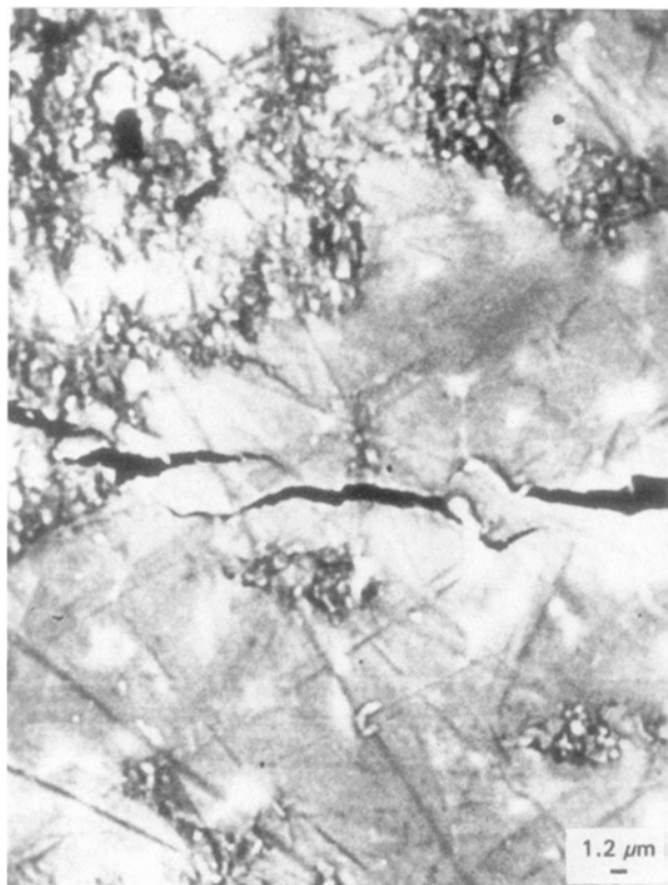
Figure 7 Scanning electron micrograph of the fatigue-crack propagation showing the occurrence of whisker-like \beta' -Sialon bridging behind the crack tip.
